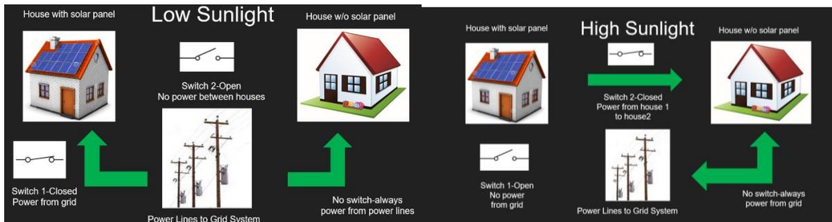
Fig. 2. Transactive energy switching concept flow charts
